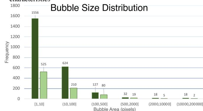
**Figure 6.** Comparison of bubble size by area and eccentricity for DI water run in the jet bubbler.
