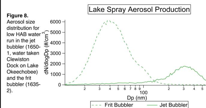
**Figure 8.** Aerosol size distribution for low HAB water run in the jet bubbler (1650-1, water taken Clewiston Dock on Lake Okeechobee) and the frit bubbler (1635-2).
