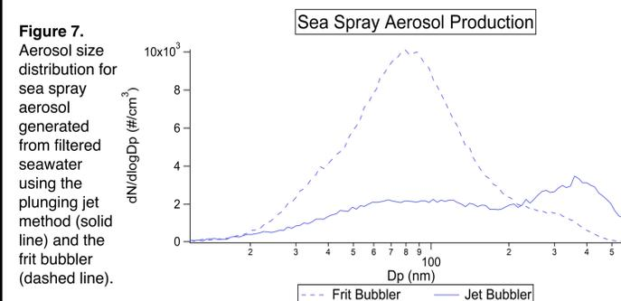
**Figure 7.** Aerosol size distribution for sea spray aerosol generated from filtered seawater using the plunging jet method (solid line) and the frit bubbler (dashed line).
